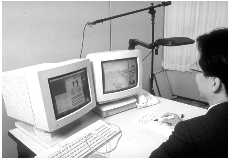
**Figure 4.2** Overview of TeamWorkStation-1 prototype
