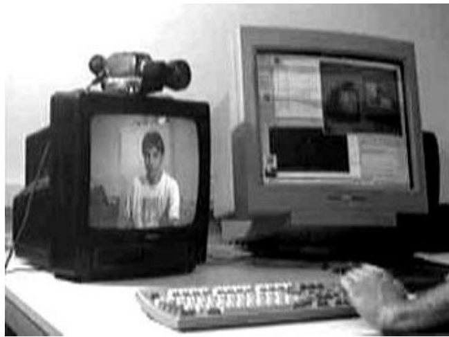
Figure 3.2 A typical configuration for an analog media space node, with a video camera, microphone, video monitor and workstation
