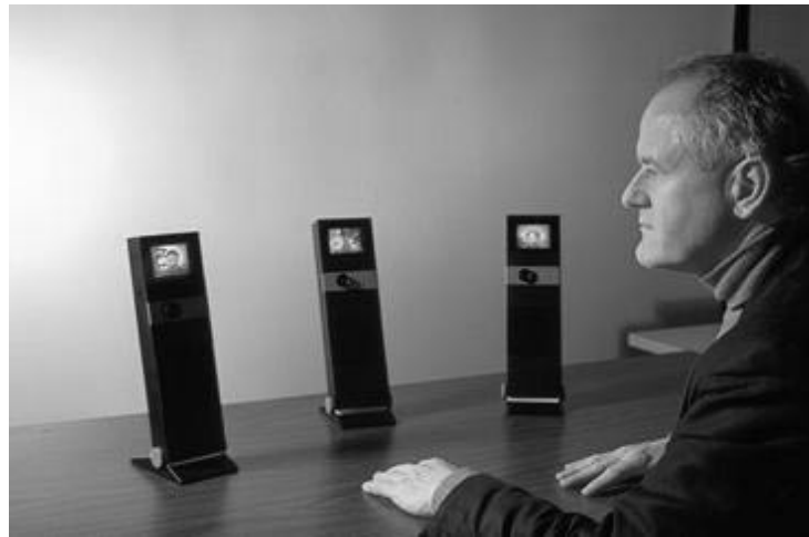
Figure 3.8 Hydra incorporates a video camera, monitor and directional microphone into a small table-top unit that can act as a proxy for distant participants of a meeting
