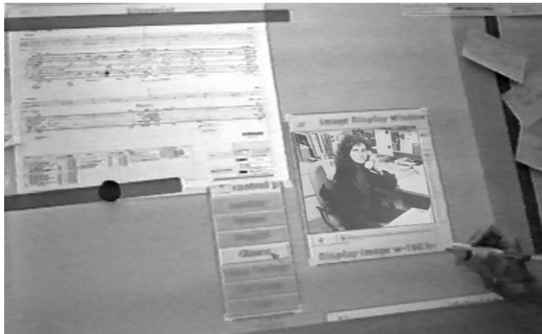
Figure 3.12 Ariel lets construction engineers access the media space and a hypermedia annotation system via paper engineering drawings. The user selects the media space option from the control section of the paper engineering drawing (upper left). Ariel projects a menu and the user selects Glance with the graphics tablet pen, which establishes a three-second connection
