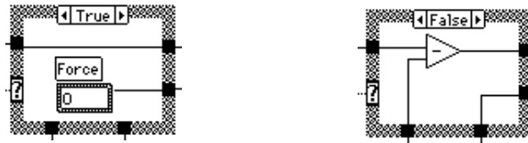
Figure 9 A LabView conditional from the rocket program, showing both arms. In the LabView environment, only one arm is visible on screen at any one time.
